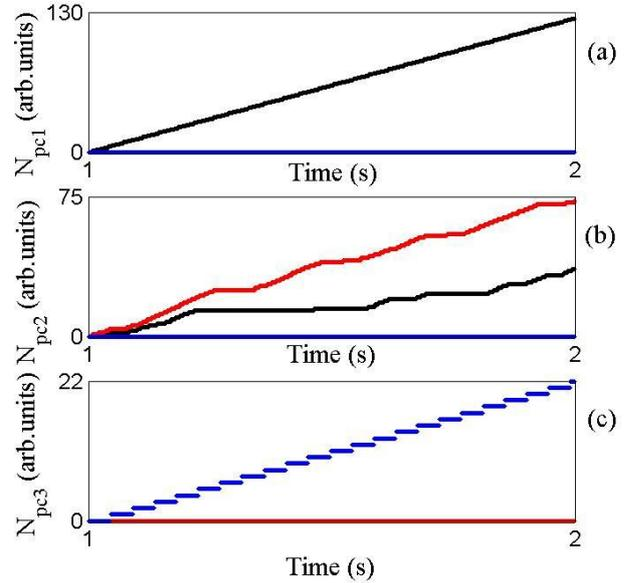
Figure 5: Number of phase coupling  $N_{pc}$  results for black - fault free, red - lubrication starving and blue line - outer bearing failure for selected fault characteristic bifrequencies (a)-(c).
