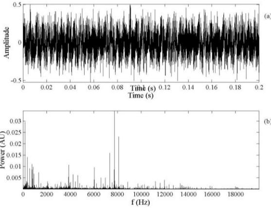
Figure 3: Envelope vibration signal for the case of fault free electrical motor. (a) Time evolution and (b) its power spectrum.
