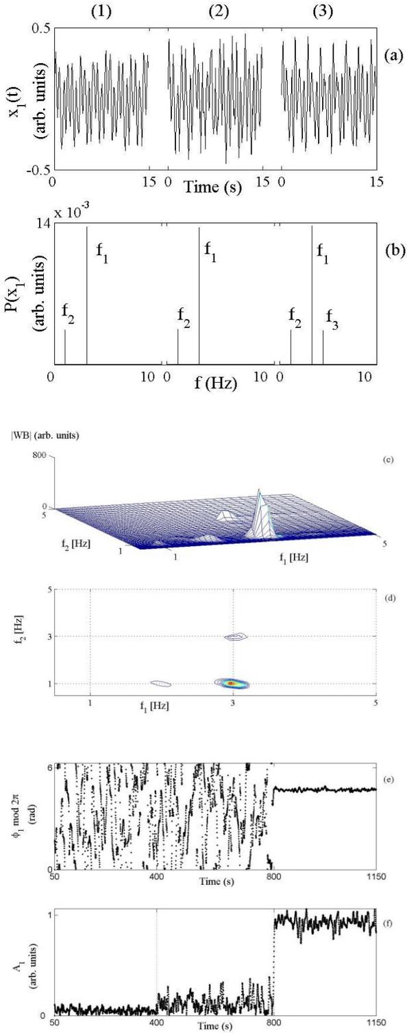
Figure 1: Generic signal  $x_1(t)$ . (a) Time evolution, (b) its power spectrum, (c) and (d) is absolute value of wavelet bispectrum and its contour plot in bifrequency domain. (e) Time evolution of biphase and (f) biamplitude.
