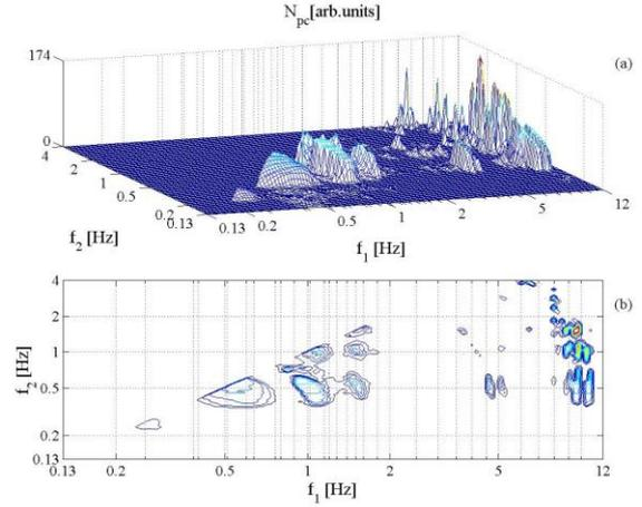
Figure 4: Number of phase couplings  $N_{pc}$  for fault free envelope vibration signal.
