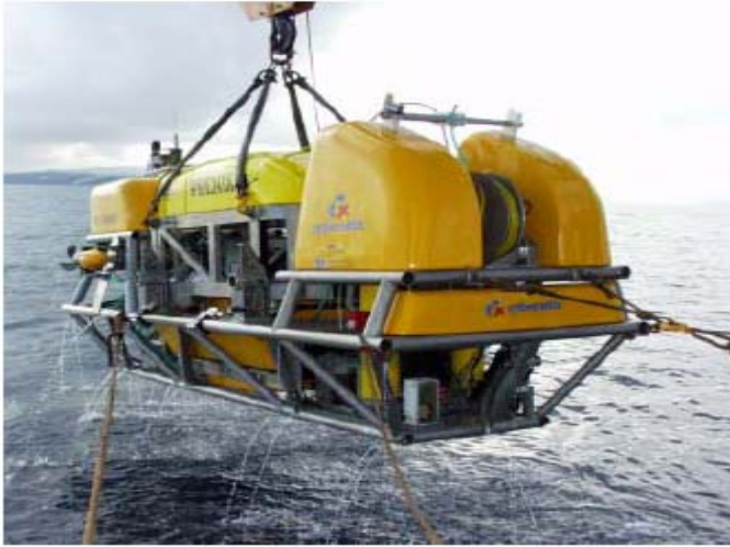
Figure 7: Example of a hybrid AUV/ROVs Swimmer (by Cybernetix).
