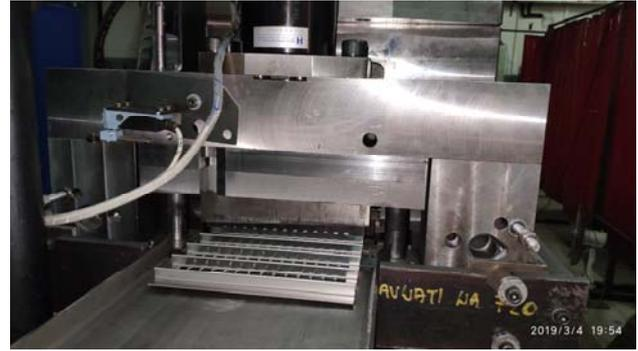
Figure 11: Detail of automatic tool for sheet metal forming.
